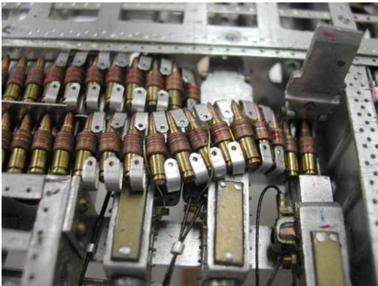
Inside the left wing you can see the .50 cal ammunition threaded into the three wing guns. Each round is machined in 3 parts?brass cartridge with copper bullet and primer and is held together with a small copper feed jacket.
