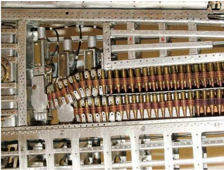
Inside the left wing you can see the .50 cal ammunition threaded into the three wing guns. Each round is machined in 3 parts?brass cartridge with copper bullet and primer and is held together with a small copper feed jacket.
